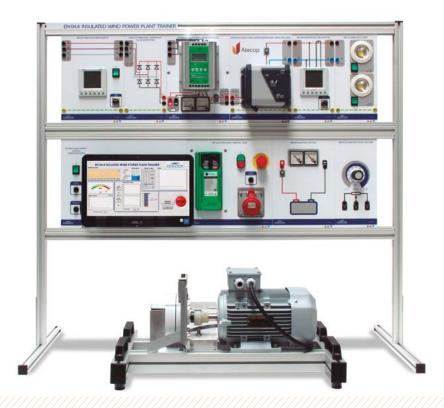
With the EN044 equipment, the behavior of a wind turbine is emulated in a practical and didactic way. An electric motor acts as the blades and bush of a wind turbine, dragging a three-phase synchronous generator of permanent magnets, which transforms the mechanical energy transmitted to the shaft into electrical energy at the output.
