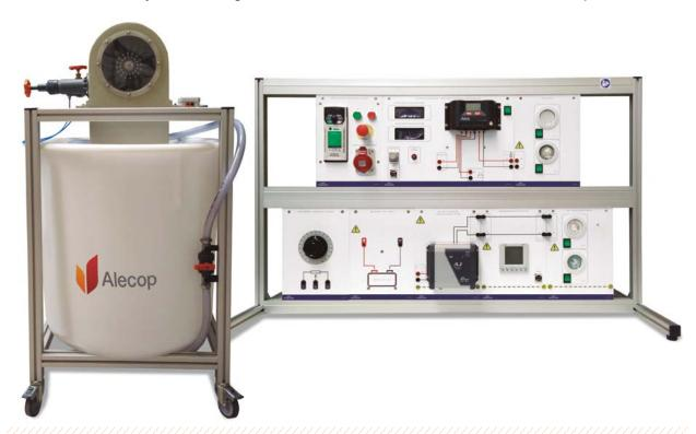
Trainer EN051 has been designed as a small-scale hydropower plant and it is equipped with a Pelton-like turbine that provides full operation along with all the other accessories that complete a standard installation.
