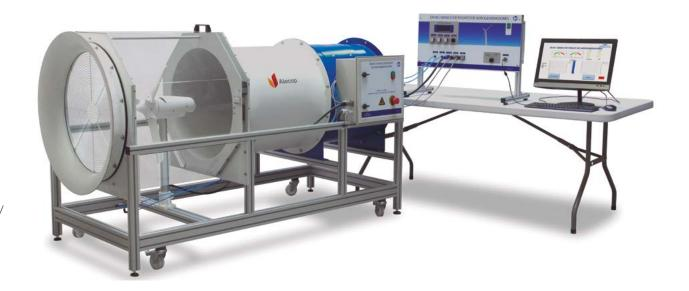
The Windmill Test-bench (EN041), is a wind tunnel of 2 meters length designed to work with windmills of less or equal to 630mm diameter. The equipment has a 612 mm windmill included, which has a torque and rotation speed measurement system.
