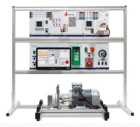
With the equipment EN042, the behaviour of a wind turbine is emulated in a practical and educational way. An electric motor operates as the turbine on a windmill moving a three-phase synchronous permanent magnet generator, which converts the transmitted mechanical energy to electric energy.
