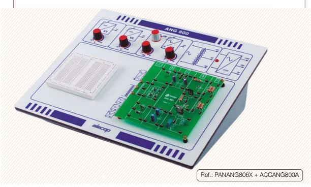
Modular trainer for the study of the basic principles of d.c. and a.c. circuits. The system is based on the ANG-800 console where the pre-constructed boards with the different systems of signal modulation and coding are placed. The console includes a prototyping area to allow for extra experiments and project work to be undertaken.
