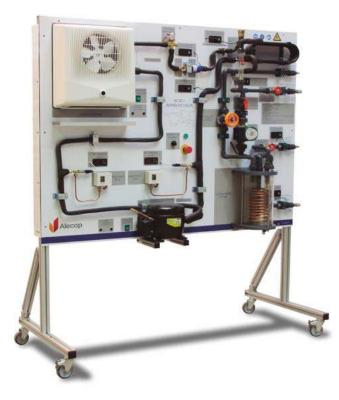
The AC031 equipment demonstrates clearly the operation of a heat pump air/water.
