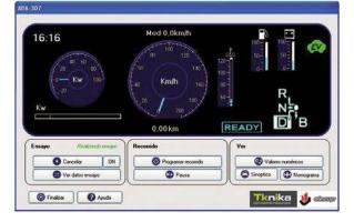
The hardware trainer is a driving simulator (gear, speed, battery charge, fuel gauge). All the actions performed on the panel are represented in the software instrument panel.
