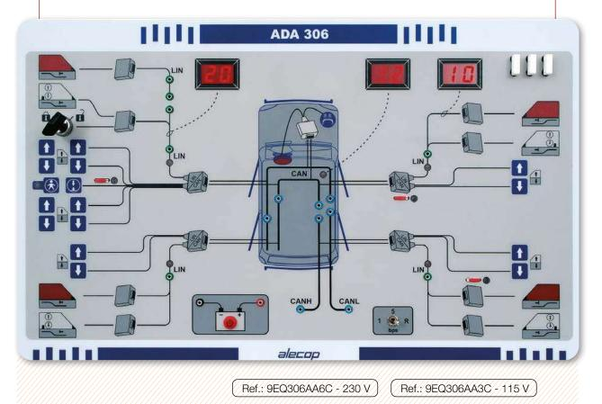
The objective of this equipment is to familiarise the student with data and multiplex networks. The information is transmitted by means of two buses: CAN (Controller Area Network, ISO 11898- 3 or ISO 11519-2 specification) and LIN (Local Interconnect Network).
