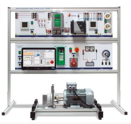
With the EN044 equipment, the behavior of a wind turbine is emulated in a practical and didactic way. An electric motor acts as the blades and bush of a wind turbine, dragging a three-phase synchronous generator of permanent magnets, which transforms the mechanical energy transmitted to the shaft into electrical energy at the output.
