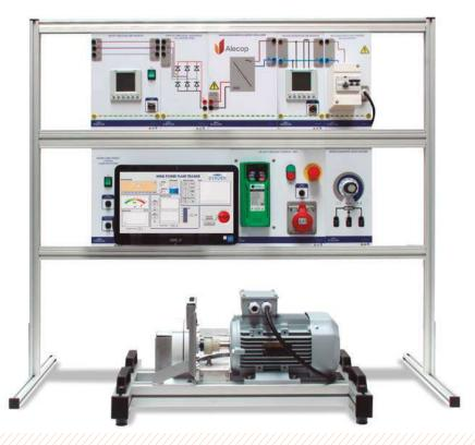
With the equipment EN042, the behaviour of a wind turbine is emulated in a practical and educational way. An electric motor operates as the turbine on a windmill moving a three-phase synchronous permanent magnet generator, which converts the transmitted mechanical energy to electric energy.
